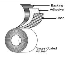
UV Stabilized LDPE Film **Backing:** Adhesive: Acrylic (A128) Liner: 53# Coated Kraft Colors: Clear Specifications: N/A Incremental widths 1/4" - 54" x 48ft
